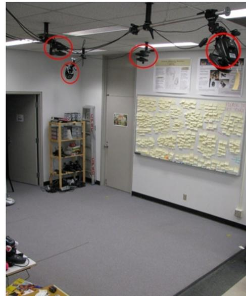
**Figure 4 – the interaction space, with some of the motion-tracking cameras in view (highlighted)**
