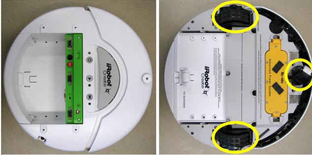
**Figure 2 – iRobot Roomba, with underside view (right) : two-wheel base and coaster highlighted**
